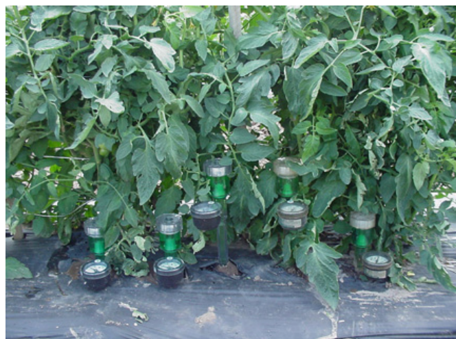
Figure 2: Tensiometers installed in a research plot of tomatoes. (Typically just one or two would be installed at one spot, not four as shown here.) ( Photo by Liz Maynard )
