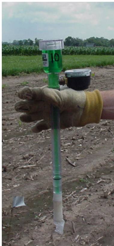
Figure 1: A tensiometer ready to be installed. The instrument is filled with water to which a green dye has been added. The ceramic tip at the bottom is covered with a plastic bag to prevent it from drying out. The plastic will be removed before installation. ( Photo by Liz Maynard )
