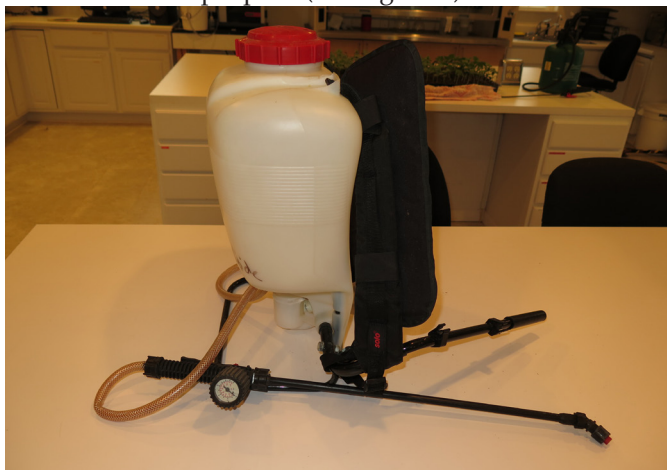
Figure 2. This backpack sprayer has a pressure gauge on the wand and a separate pump handle so that pressure can be maintained while spraying. (Photo by Dan Egel)
