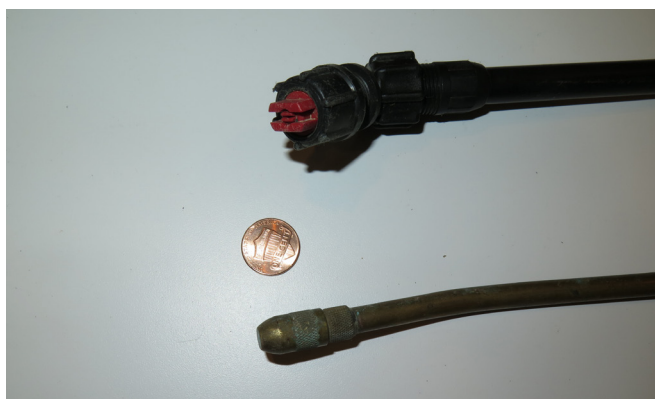
Figure 3. The top nozzle is a flat fan nozzle designed for pesticide applications. The bottom multi-purpose nozzle may be adjusted from a thin stream to a wide spray and may be changed accidentally during a pesticide application. (Photo by Dan Egel)
