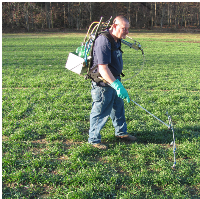
Figure 4. Here the use of a backpack CO 2 sprayer is demonstrated. Advantages of this sprayer are the CO 2 propellant that allows a consistent spray and a boom of 4 nozzles that makes applications easier and more effective. (Photo by Dan Egel)
