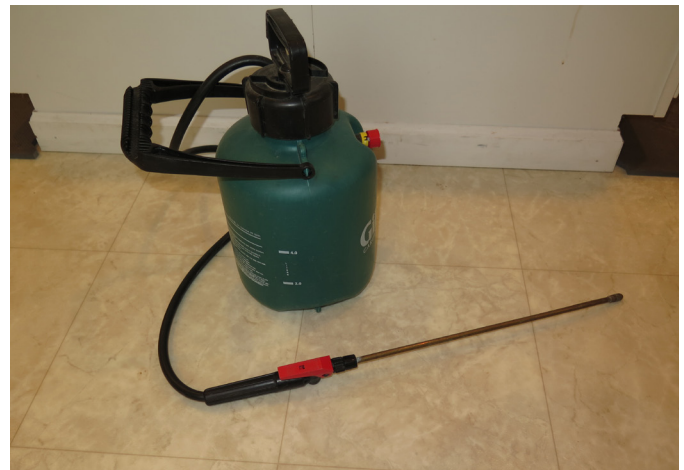
Figure 1. The common hand sprayer may be purchased at the local hardware or garden store. Note that this one has a quick release valve. (Photo by Dan Egel)
