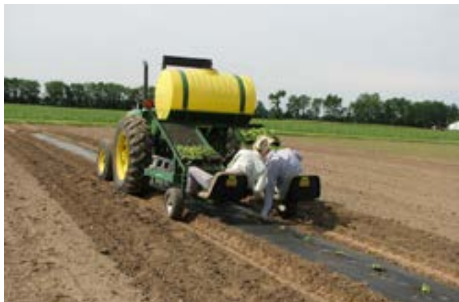
Figure 4. Waterwheel transplanters are commonly used for vegetables on plastic-covered beds. (Photo by K. Freeman)
