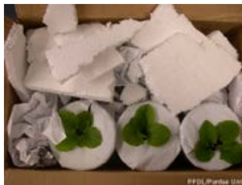
Figure 8. Use styrofoam, packing peanuts, or crumpled newspaper inside a crush proof box to protect the sample during shipment.
