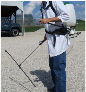
Figure 2. This backpack sprayer has three nozzles on a boom and a hand-pump that can be worked constantly.
