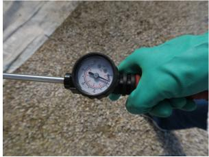
Figure 3. A gauge on the handle of the backpack sprayer allows one to constantly monitor pressure.
