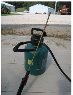
Figure 1. A typical garden sprayer with an adjustable nozzle and hand pump is not suitable for applying most commercial pesticides.
