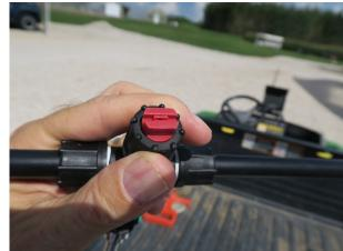
Figure 4. This flat fan nozzle provides constant output.
