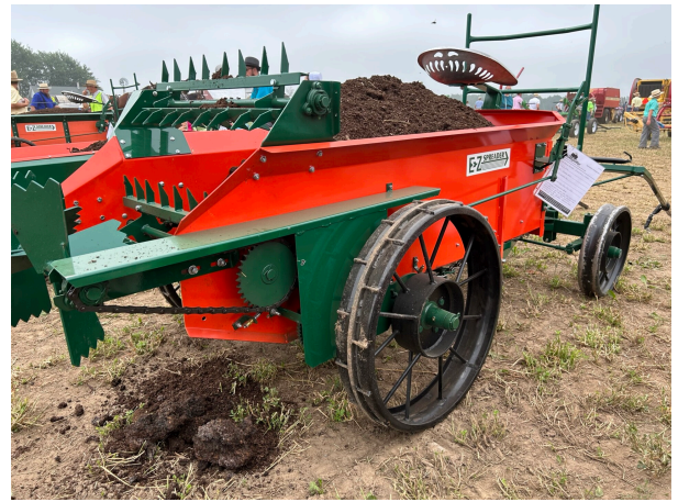
Figure 4. Ground-driven manure spreader by EZ Spreader LLC. demoed at Horse Progress Days in Shipshewana, IN (Photo by Moriah Bilenky).
