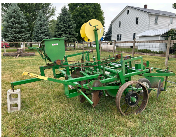
Figure 8. Horse-drawn plastic mulch layer by EZ Trail Manufacturing (Photo by Moriah Bilenky).
