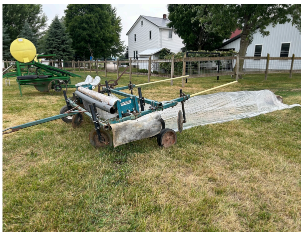
Figure 9. Pull-type low tunnel maker by Buckeye Tractor Co (Photo by Moriah Bilenky).
