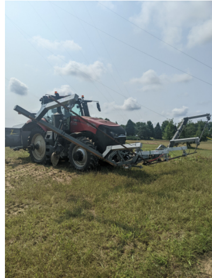
Figure 9. A weed zapper mounted to the front of a large tractor (Photo by S.L. Meyers).
