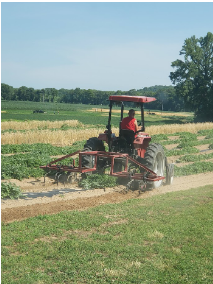
Figure 4. A tractor-mounted S-tine cultivator removes small weeds from row middles of plasticulture watermelon (Photo by J. Arana).
