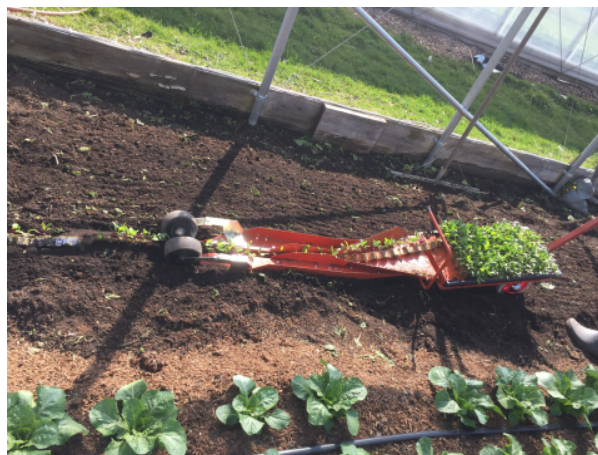
Figure 3. Paper pot transplanter saves labor, especially when transplanting closely-spaced seedlings (Photo by E. Maynard).
