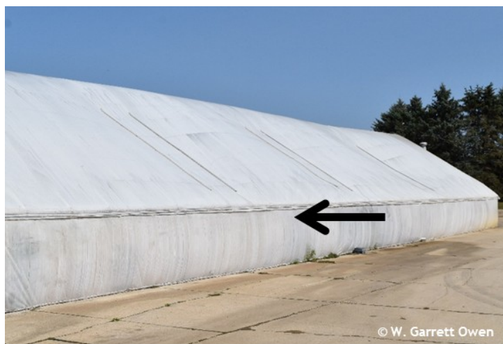
Figure 16. Seasonal application of greenhouse whitewash utilized to limit solar ambient light into the greenhouse environment, thereby reducing daily light integral.
