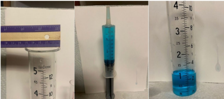
Figure 2. Follow these simple steps to check the accuracy of a rain gauge
